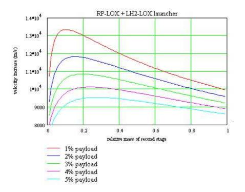
Firstly, we notice that in all cases the optimum combination is a second stage four to five times lighter than the first stage: thus for the two-stage Saturn V used to launch Skylab in 1973, the first stage mass was 2286 t (t for metric ton) while the second stage mass was 491 t.
