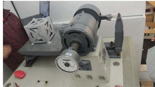
Figure 23. Non-standard CubeSat coupled at Vibration test bench. Source: Cortés-García *et al.* (2019).
