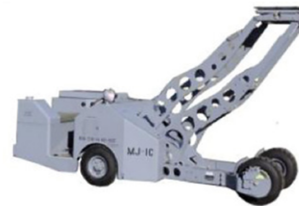
Figura 17. Aircraft Aerial Munitions Lift Trucks/Aircraft Bomb Loaders, MJ-1C (2) replaces MJ-1A & MJ-1B; P/N: 8141050-70 (NSN: 1730-01-491-1557), de [15]
