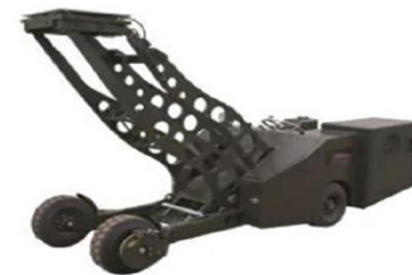
Figura 18. Aircraft Aerial Munitions Lift Trucks/Aircraft Bomb Loaders, MJ-1E P/N: 050025-100 (NSN: 1730-01-536-6388) Electric Motor Driven, de [15]
