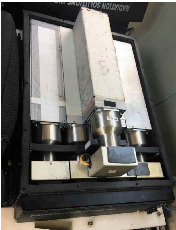
Figure 2. Example of a Crystal Box installed in an aircraft. Source: E. Camara, October 2016. Author's private collection
