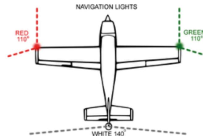
**Figure 6.** Aircraft position/navigation lights. Available from: <https://learntofly.ca/aircraft-navigation-lights/>
